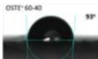
Fig. S1. Measured hydrophobicity of prepared monomer stock solution.
