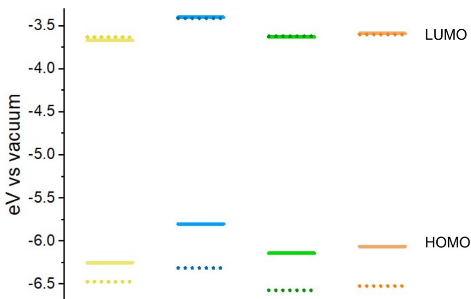
Figure S6. Energy diagram of experimental (solid lines) and computed (dotted lines) energy levels of HOMO and LUMO orbitals of compounds 1 (yellow), 2 (blue), 3 (green), and 4 (orange).
