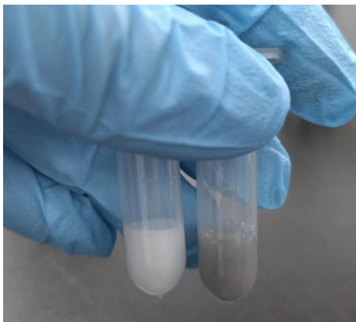
Figure S3 The solutions mixed with \text{HfO}_2 powders purchased from Aladdin (Left) and prepared by hydrothermal method (Right).
