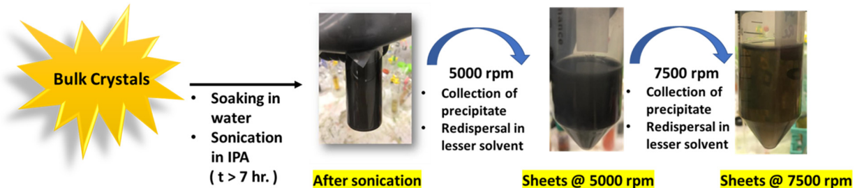
Figure S3. Schematic representation of the liquid phase exfoliation of \text{MnIn}_2\text{Se}_4 crystals. The sheets isolated at the centrifugation speeds of 5000 and 7500 rpm were taken for further studies.
