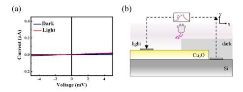
**Figure S2.** (a) *I-V* characteristics and (b) schematic diagram of the device structure for Pt/Cu<sub>2</sub>O/Si/Pt under asymmetrical light illumination.
