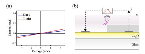
**Figure S1.** (a) *I-V* characteristics and (b) schematic diagram of the device structure for Pt/Cu<sub>2</sub>O/Pt under asymmetrical light illumination.
