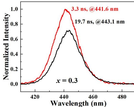
**Fig. S3.** The decay-associated spectra, as well as the peak positions and lifetimes, of the  $\text{Cd}_{0.7}\text{Zn}_{0.3}\text{S}/\text{ZnS}$  QDs obtained from ns time-resolved PL spectra.
