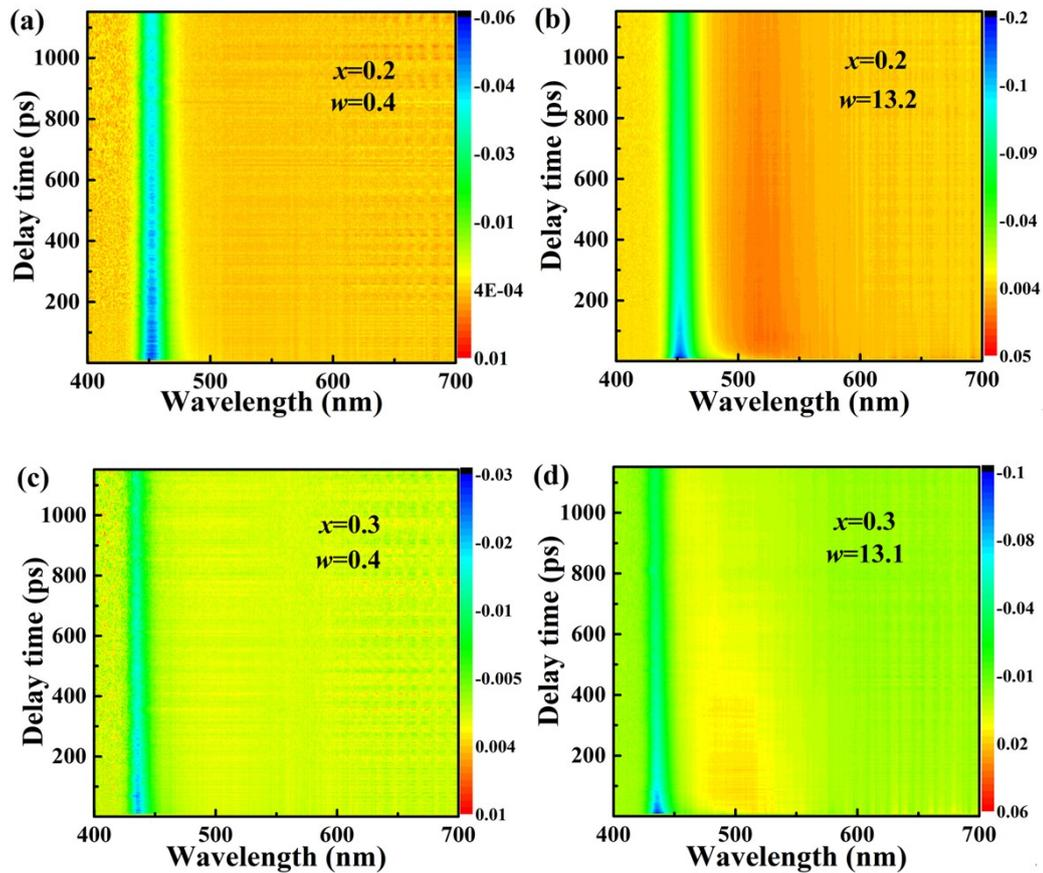
**Fig. S5.** The spectral 2D contours of (a) (b)  $\text{Cd}_{0.8}\text{Zn}_{0.2}\text{S}/\text{ZnS}$  and (c) (d)  $\text{Cd}_{0.7}\text{Zn}_{0.3}\text{S}/\text{ZnS}$  QDs at representative low and high pump fluences.
