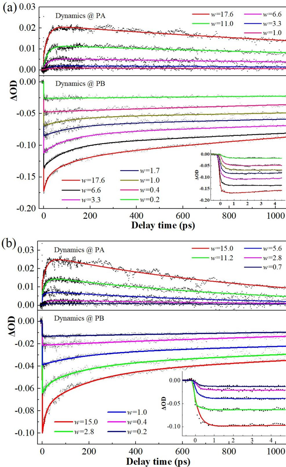
Fig. S7. Dynamics of (a) Cd<sub>0.8</sub>Zn<sub>0.2</sub>S/ZnS and (b) Cd<sub>0.7</sub>Zn<sub>0.3</sub>S/ZnS QDs probed at PB and PA regions under different pump fluences. The inserts shows the rising edge of the dynamics.
