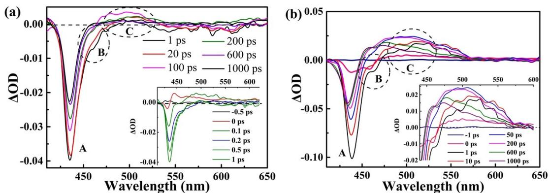
**Fig. S6.** Transient absorption spectra of  $\text{Cd}_{0.7}\text{Zn}_{0.3}\text{S}/\text{ZnS}$  QDs at different delay time at (a) low ( $w=1.0$ ) and (b) high ( $w=15.0$ ) pump fluences. The inserts in panel (a) and (b) show the TA spectra before and after 1 ps, respectively.
