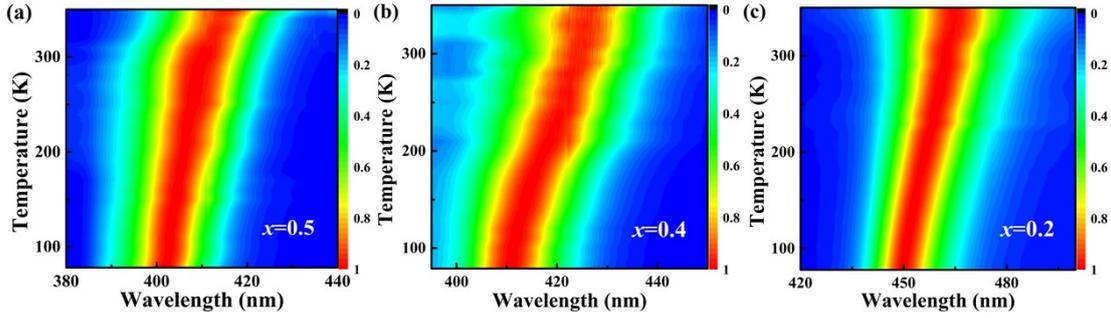
**Fig. S1.** (a)-(c) Steady-state PL spectral contours of  $\text{Cd}_{1-x}\text{Zn}_x\text{S}/\text{ZnS}$  QDs ( $x=0.5$ ,  $0.4$ , and  $0.2$ ) measured at the temperatures range from 80 to 350 K.
