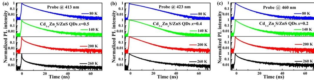
**Fig. S2.** (a)-(c) Time-resolved PL dynamics of  $\text{Cd}_{1-x}\text{Zn}_x\text{S}/\text{ZnS}$  QDs ( $x=0.5$ ,  $0.4$ , and  $0.2$ ) at 80, 140, 200, 260 K probed at corresponding emission peaks.
