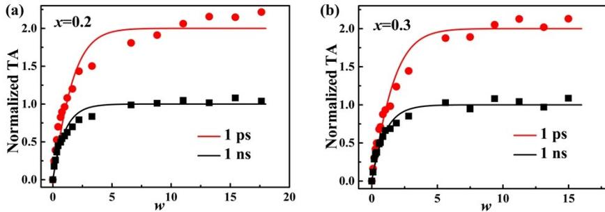
**Fig. S4.** Normalized transient photoinduced bleach signals for  $\Delta S_{t_0}$  (red circles) and  $\Delta S_{t_L}$  (black squares) in (a)  $\text{Cd}_{0.8}\text{Zn}_{0.2}\text{S}/\text{ZnS}$  and (b)  $\text{Cd}_{0.7}\text{Zn}_{0.3}\text{S}/\text{ZnS}$  QDs as a function of average number of excitons per QD. The solid lines are fits according to the model described above.
