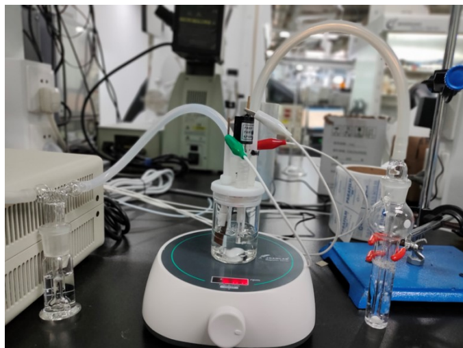
Fig. S1. Experimental apparatus of the electrochemical reduction of \text{N}_2 to \text{NH}_3 .
