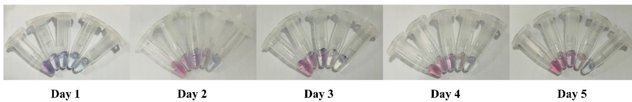
Fig. S5. Storage stability performance. Color change of AuNPs solution in five days.
