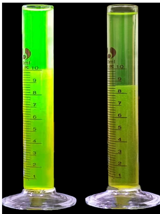
Fig. S6 Response characteristics of fluorescent hydrogels to Hg^{2+} . Volume changes of the fully swelled fluorescent hydrogel after soaking in 3.0 \times 10^{-4} \text{ mol} \cdot L^{-1} NaCl solution (left) and 1.0 \times 10^{-4} \text{ mol} \cdot L^{-1} Hg(NO_3)_2 solution (right) for 30 min.
