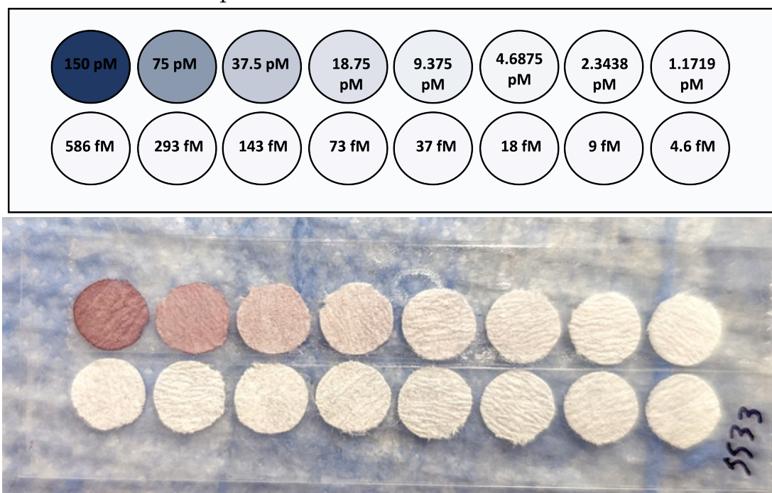
Figure S18. Concentrations of SERS and SERRS nanoparticle colloidal solutions applied onto the filter paper substrate for dilution series.
