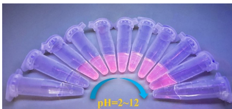
Fig.S4. Images of Eu-MOF/BA in the solution of different pH under the UV lamp at 265 nm.
