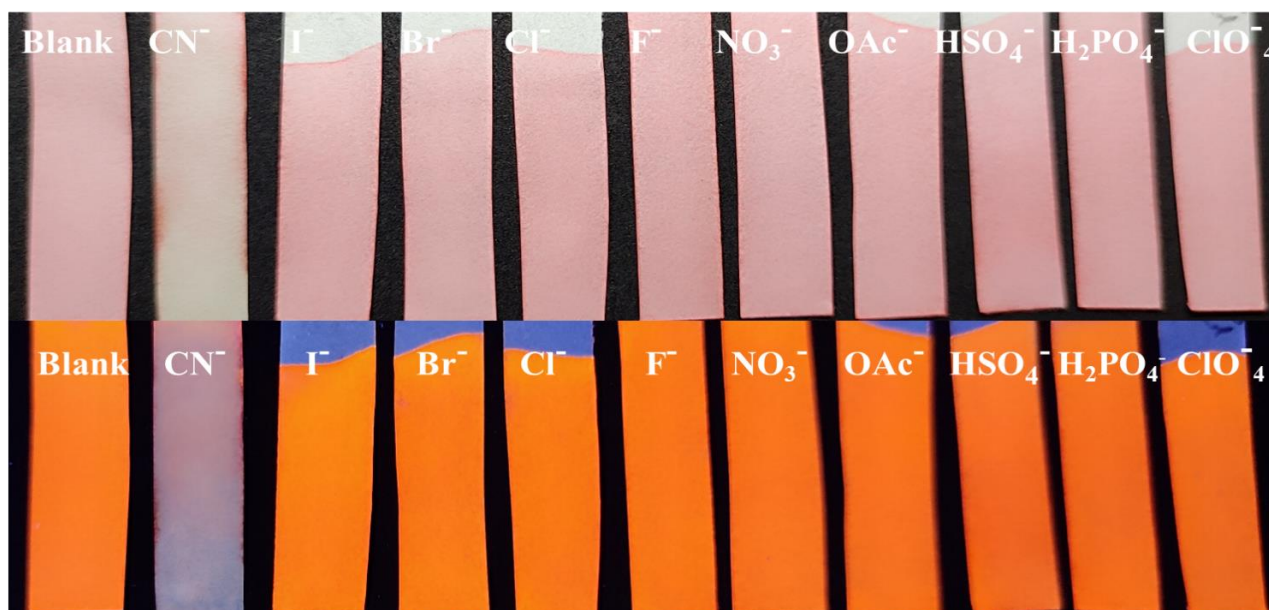
Figure S14. Paper strip based selectively detection of \text{CN}^- ion with the probe NDI 1 , over other anions used by naked eyes a) under visible light and b) under 365 nm UV light.
