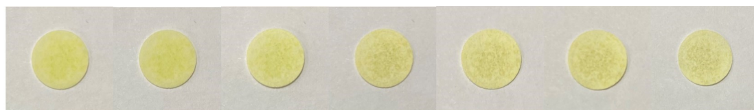
Fig. S12. The color response of the paper-based biosensor after storing at room temperature for seven days.
