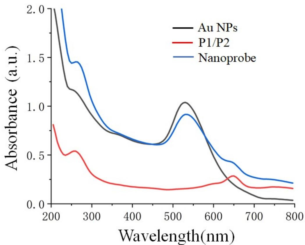
**Fig. S4.** The UV-vis spectrum of the Au NPs, P1/P2 hybrid and Au-DNAzyme nanoprobe.
