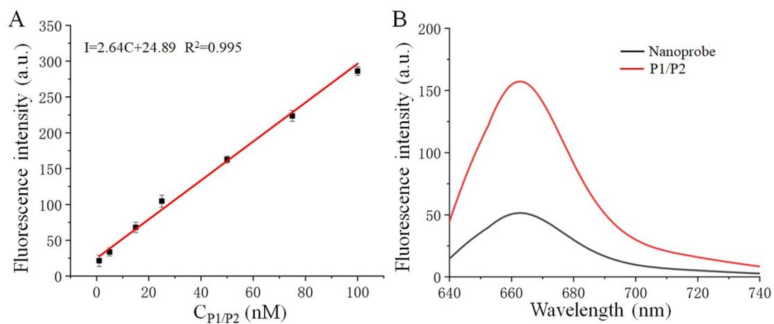
**Fig. S5.** (A) The standard linear calibration curves of the P1/P2 hybrid; (B) The fluorescence spectra of the P1/P2 hybrid before and after were immobilized on the Au NPs in liquid supernatant. Error bars were derived from n=5 experiments.
