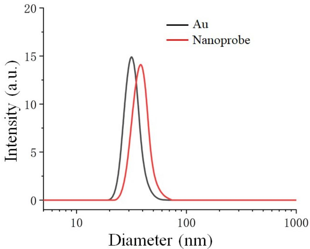
**Fig. S2.** DLS of Au NPs and Au-DNAzyme nanoprobe.
