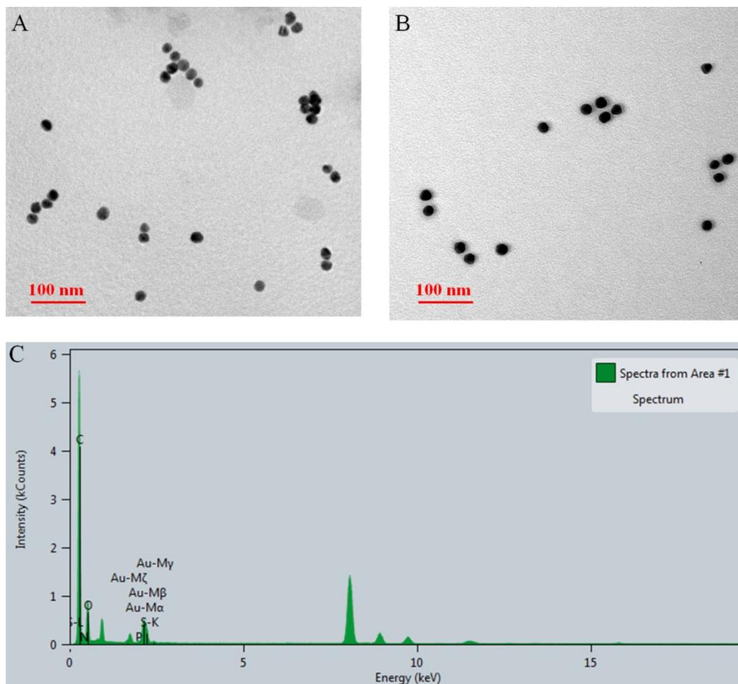
**Fig. S1.** (A) TEM of Au NPs; (B) TEM of Au-DNAzyme nanoprobe; (C) Energy Dispersive X-Ray Spectroscopy of Au-DNAzyme nanoprobe.
