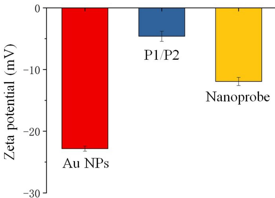
**Fig. S3.** Zeta potential analysis of Au NPs, P1/P2 hybrid and Au-DNAzyme nanoprobe. Error bars were derived from N=5 experiments.
