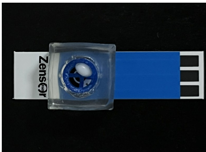
Fig. S1 Image of the SPE, PDMS chamber (including plastic interlayer), and magnetic rotor.
