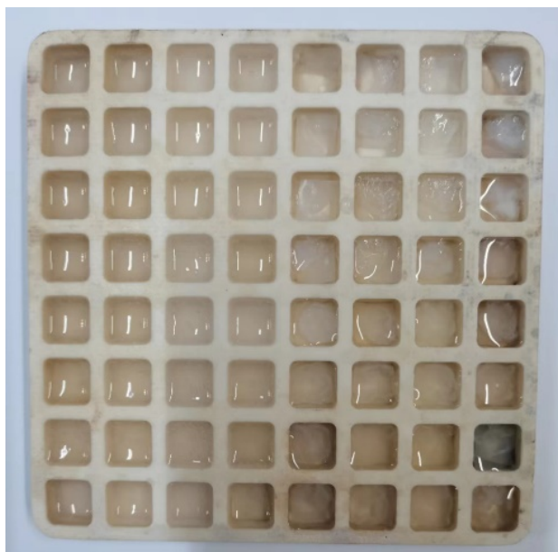
Fig. S5. Multiwall Teflon reactor, contains 8*8 holes (1 cm*1 cm, 0.8 cm depth), corresponding to each small square respectively.
