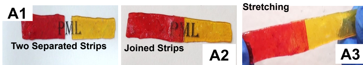
Figure S10: Demonstration of self-welding ability of PTE-0.5, (A1) two separated strips, (A2) A1 after completion of welding, (A3) A2 strip under stretched conditions.
