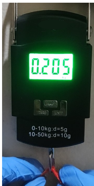
Figure S13: A remolded strip of PTE-0.5 stretched against 205 gm load.
