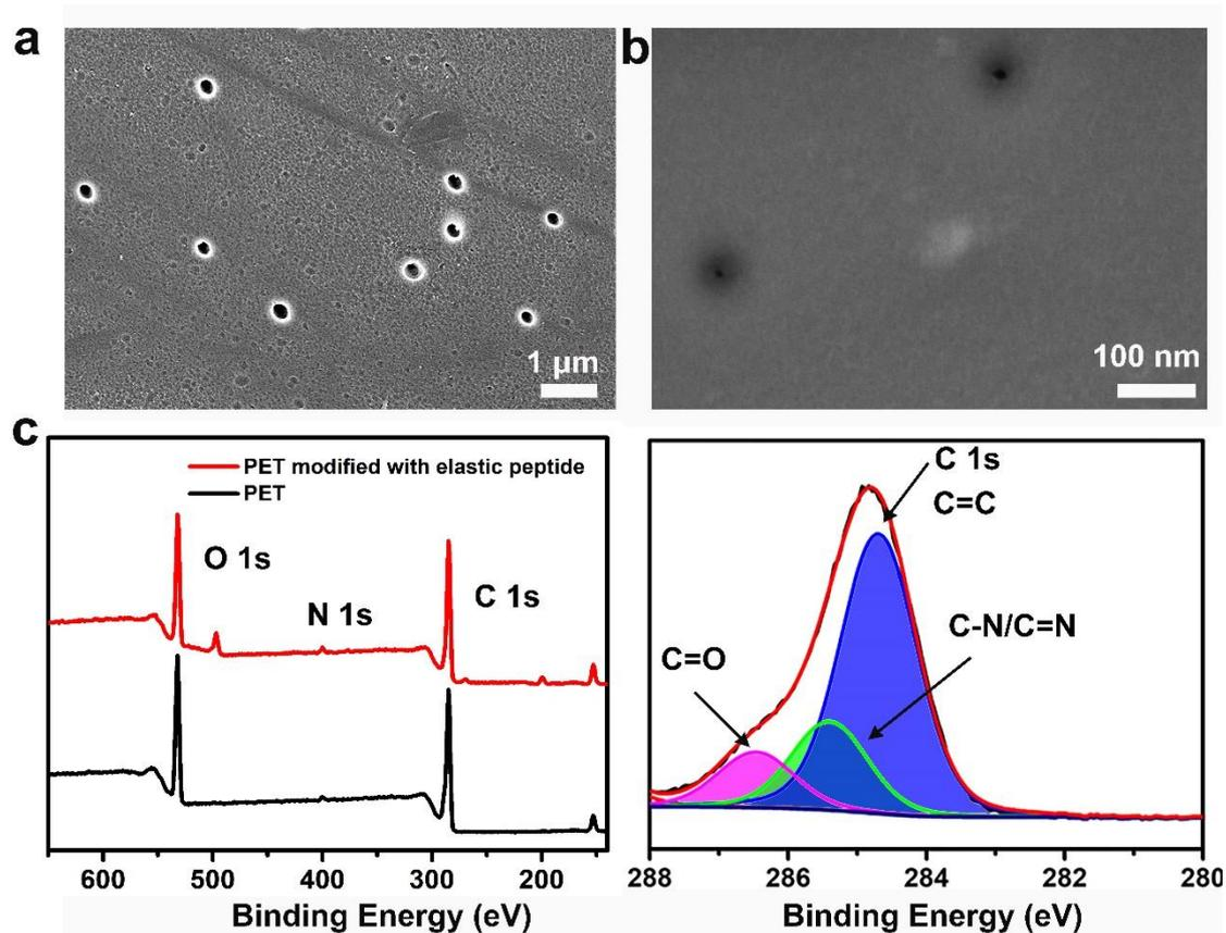
**Fig. S1** Characterization of PET membrane. a, b, TEM of pore size of the large opening (a) or small opening (b) of PET membrane nanochannel. c, XPS measurement of PET membrane before (blank line) or after (red line) modified with ES peptide.
