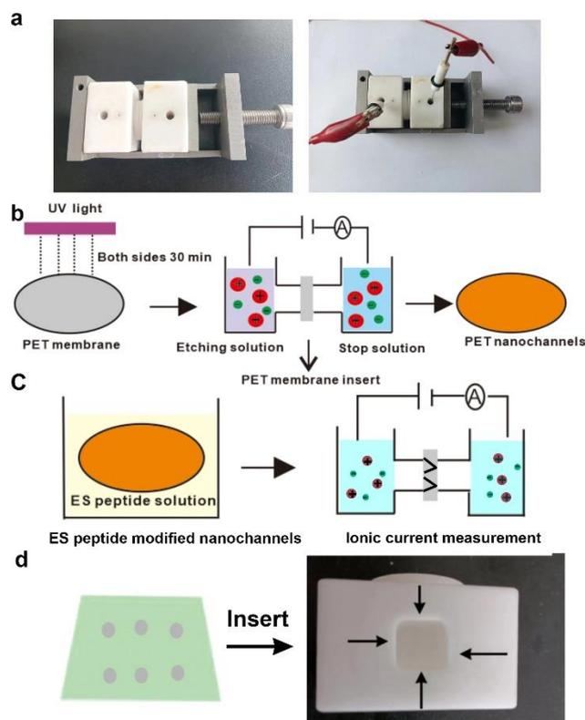
**Scheme S1** a, The schematic diagram of the etching and measurement device. b, The etching process of multiple conical nanochannels. c, The preparation of ES peptide-modified PET nanochannels. d, The strategy for living cells inserted into the modules.
