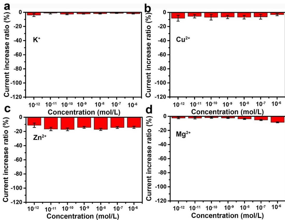
**Fig. S2** Concentration-dependent ionic current increase ratio (at -2 V) of the ES peptide-modified PET nanochannel membrane in 0.01 M NaCl solution upon a series of  $K^+$  (a),  $Cu^{2+}$  (b),  $Zn^{2+}$  (c) and  $Mg^{2+}$  (d).
