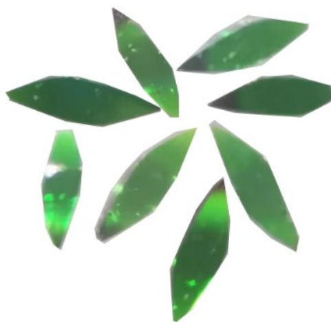
Figure S10. Photograph of the compound CoTBT after immersion in 20M NaOH for 5 days at room temperature.
