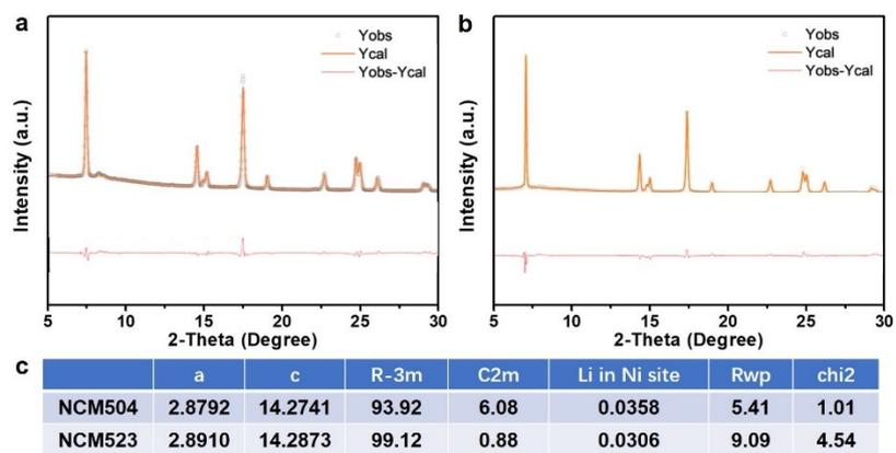
**Fig. S3.** XRD Rietveld refinement of cathodes. a, NCM504 cathode; b, NCM523 cathode; c, refinement parameters.
