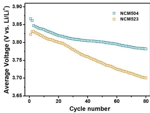
**Fig. S4.** Average voltage of NCM504 and NCM523 in half cell.
