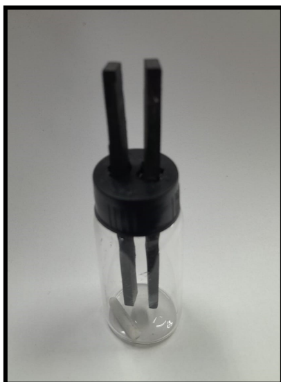
Figure S2. Reaction flask and graphite electrodes used in the electrochemical reactions.
