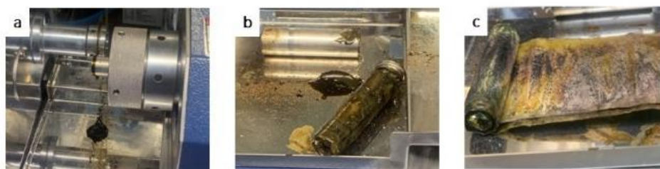
Fig. S2 Cell disassemble illustrating the electrolyte residue leakage during disassemble (a), cell roll and electrolyte residue out of the case (b), and the electrode surfaces (c).
