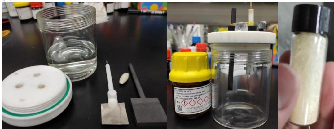
Figure S1. The set up of electrochemical reaction. (a) Equipment of standard reaction; (b) Equipment of gram-scale reaction.
