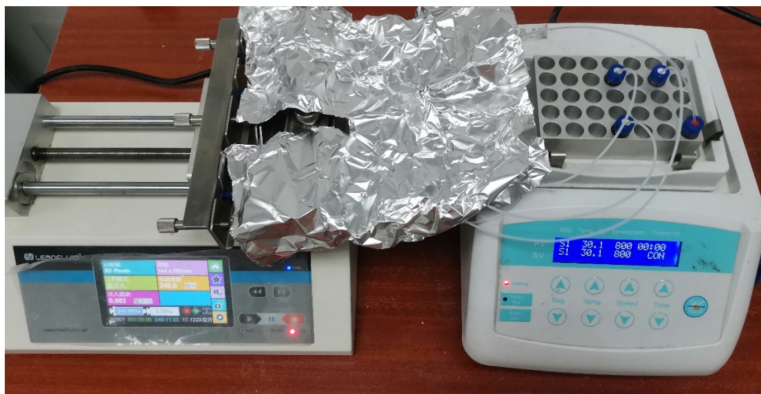
Figure S1. Experimental facility for enzymatic reactions with H 2 O 2 dosing.
