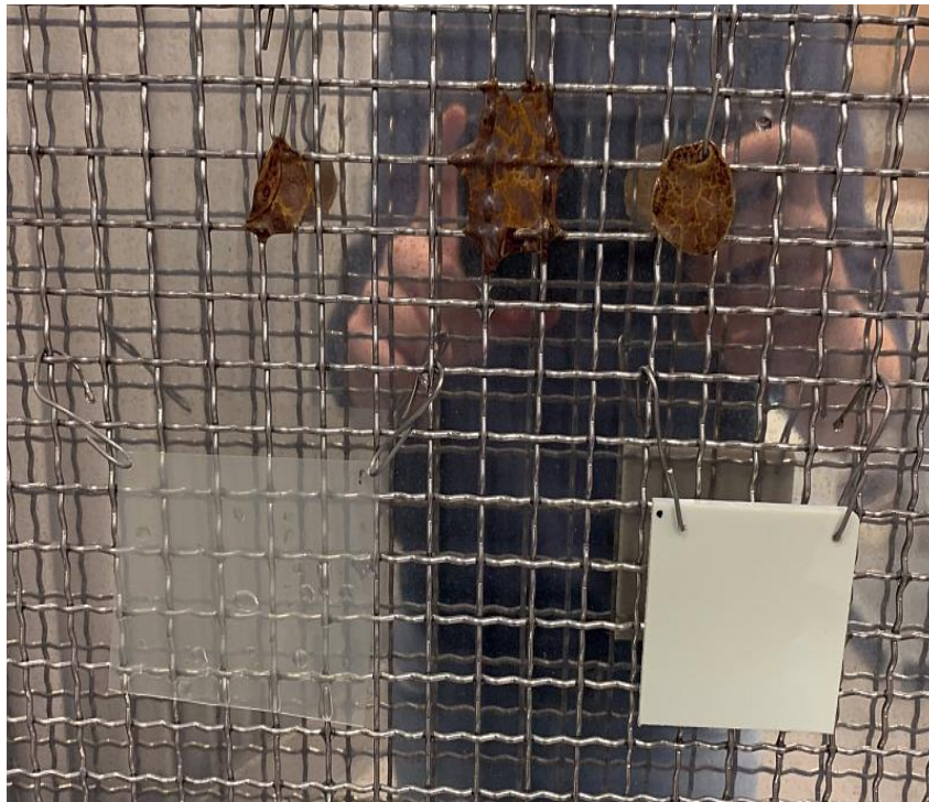
Figure S 18: Photo of the thioester samples (top row) and the all-ester reference samples (lower row) PET (left) and PBT (right) before and after weathering.
