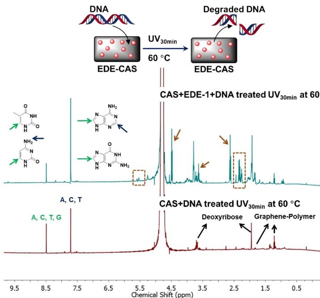
**Figure S1.** Proof of degradation by NMR:  $^1\text{H}$ -NMR studies on CAS+DNA (lower) and EDE-CAS+DNA (upper) samples treated by 360 nm of UV irradiation for 30 min at a temperature of 60 °C. Extra peaks generated by EDE-1 activation (upper spectra) indicates the role of EDE-1 in DNA degradation. 400 ng of pBR322 DNA (100 ng/ $\mu\text{L}$ ) was used for NMR study.
