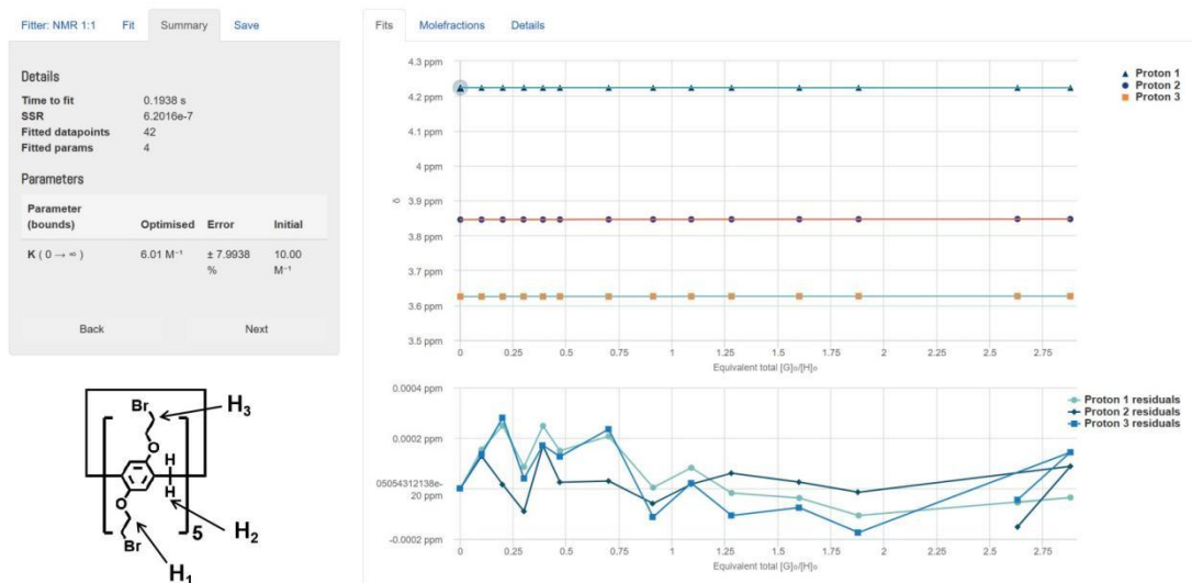
Fig. S19 A plot of the resonance downfield shifts of H 1 , H 2 and H 3 of BrP5 versus [\text{MBT}] / [\text{BrP5}] . The data were fitted to a 1:1 binding model to give K = 6.01 \pm 0.48 \text{ M}^{-1} . All solid lines were obtained from non-linear curve-fitting to a 1:1 binding model using the www.supramolecular.org web applet.
