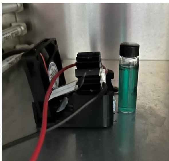
Figure S12. Setup used for LED irradiations at \lambda_{\text{max}} = 625 \text{ nm}
