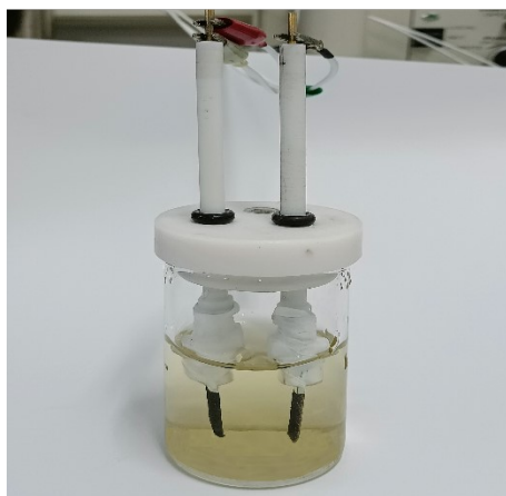
Fig. S12 The photograph of an electrochemical cell for the water-glucose co-electrolysis system.
