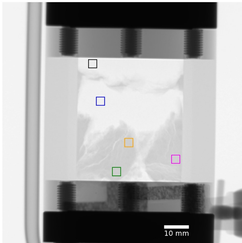
Figure S5. Full frame neutron radiograph of Sample 2 in a stainless steel cell. This image comprises 250 seconds of total exposure, created by averaging 50 \times 5s -radiographs for reduced noise levels. Coloured squares correspond to regions of interest (ROI), the time evolution of these is plotted in Figure S6.
