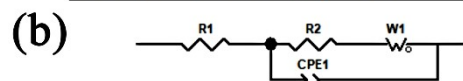
Fig. S5 (a) Impedance list of the charge-discharge cycle, (b) equivalent circuit.
