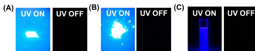
Figure S3. Photographs of compound 1 in solid state (A, crystal; B, powder) and solution state (C, dichloromethane solution) under 365 nm UV light and after removal of the UV light.
