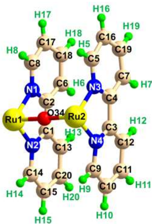
Fig. S4 Ball and stick representation of organic-hybrid-ruthenium \{\text{Ru}_2\text{O}(\text{bpy})_2\} centre linkage in cluster 1.
