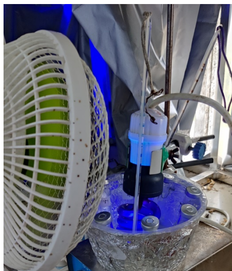
Figure S2 Reaction setup with a fan to maintain the temperature below 35 °C
