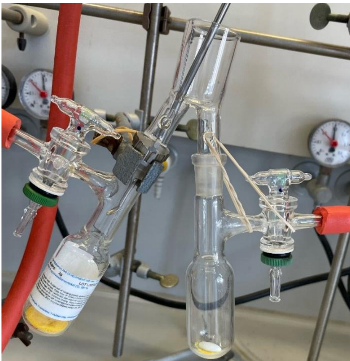
Figure S3. Use of “argon pants” for the transfer of air-sensitive compounds such as \text{Ni}(\text{cod})_2 . The reaction and reagent flasks are connected via a glassware with two legs and an open top. Argon is run through both Schlenk flasks continuously to ensure an inert atmosphere. This technique allows weighing of air-sensitive compounds without use of a glovebox.
