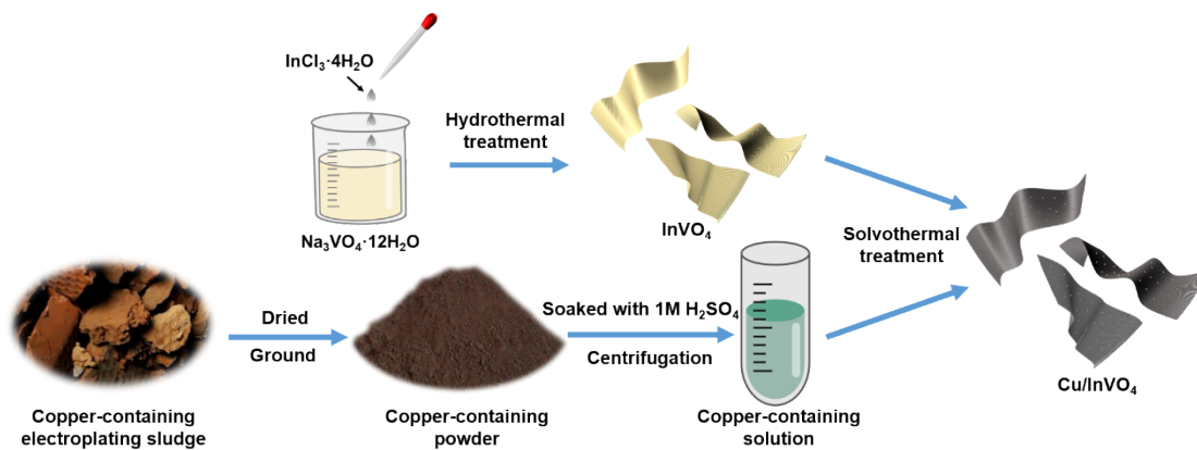
Scheme S1. Schematic diagram of the process of extracting copper from electroplating sludge to prepare Cu/InVO 4 .
