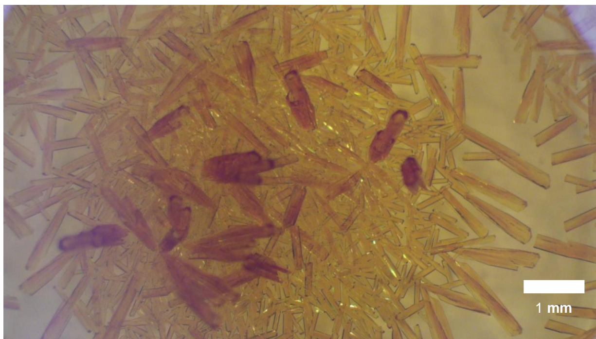
Figure S6. Digital image of as-grown Trip2Sez1Tez-I in NMP showing the rod/needle crystal morphology.
