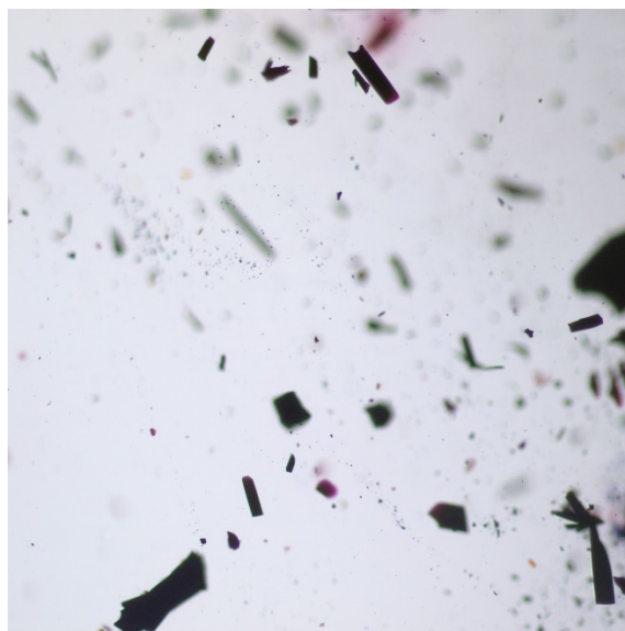
Figure S1 – Pictures of the single crystals of complex 2 used for X-ray diffraction studies.
