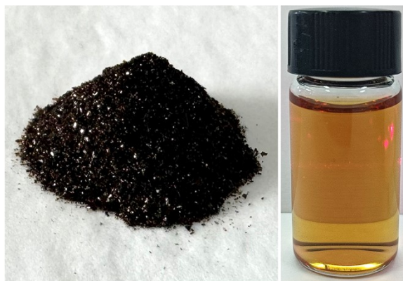
Fig. S2 Photographs of as-prepared C_{60}(OH)_{24} powder and its solution in water ( 0.5 mg\ mL^{-1} ) showing no obvious Tyndall effect.
