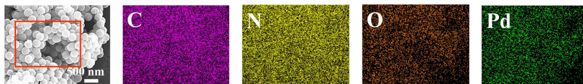
Fig. S12 SEM-EDX elemental mapping images of Pd@DhaTAPB-COOH .
