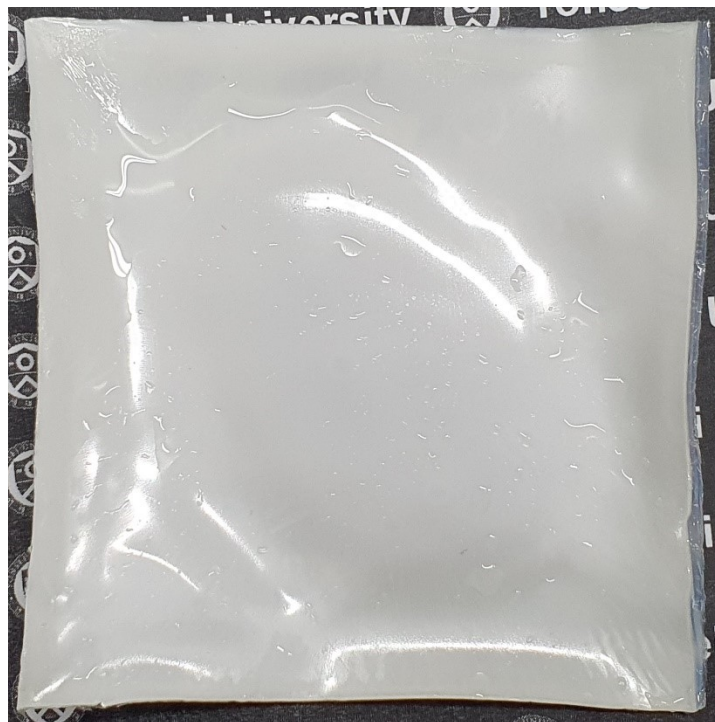
Figure S2. Photo of large area ( 10 \times 10 \text{ cm}^2 ) MI/PSF membrane prepared by reverse method.
