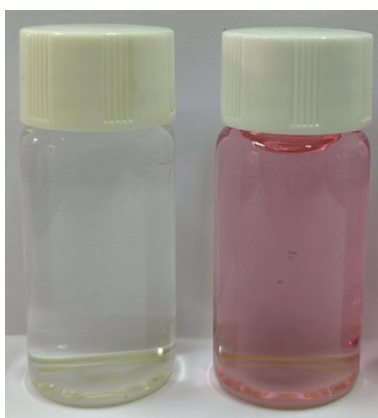
Fig. S7. Optical pictures of the co-oxidation of 4-AAP and phenol to APBQ using S-COF (left) and HRP@S-COF (right).
