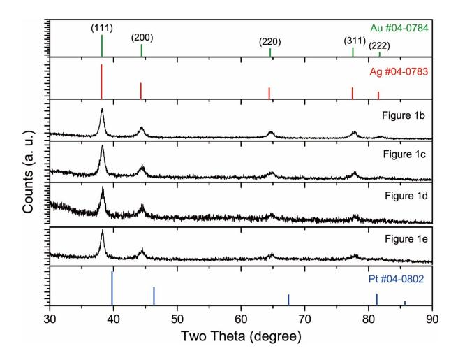
**Figure S1.** XRD patterns of products shown in Figure 1. Standard peaks of Au, Ag, and Pt are provided for reference.
