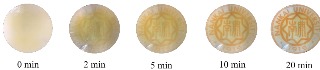
Figure S13. The printing effect of prepared printing paper at different irradiation time.
