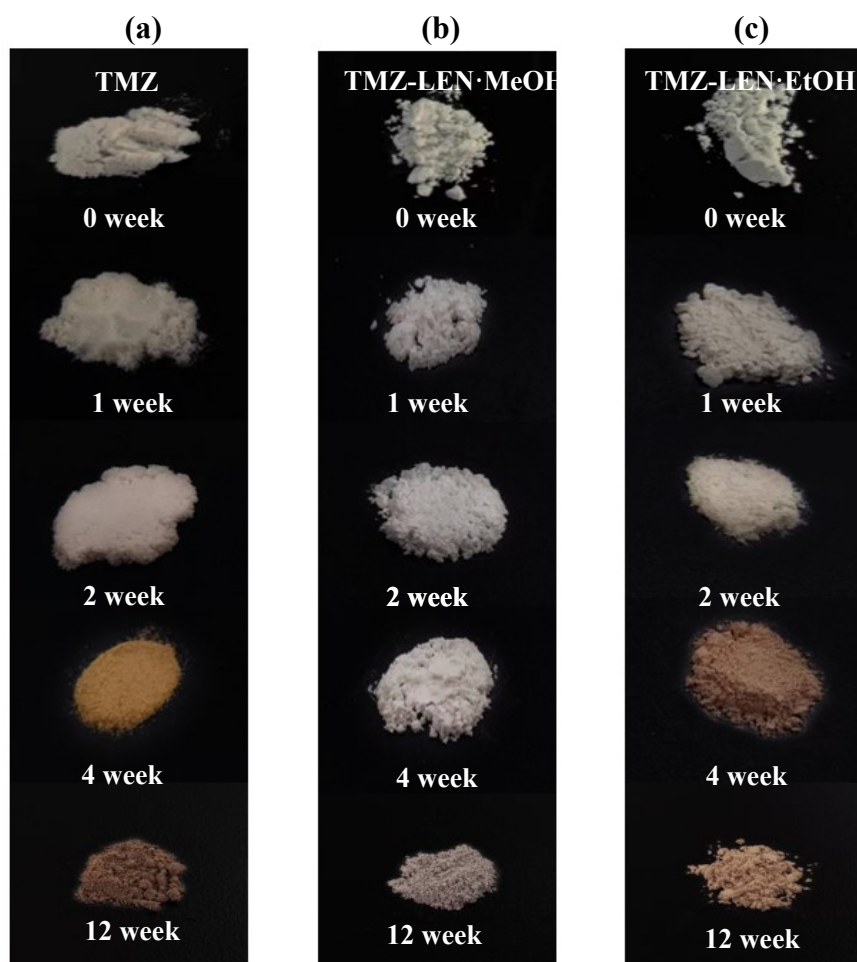
Fig. S4 Color comparison of pure (a) TMZ, (b) TMZ-LEN·MeOH and (c) TMZ-LEN·EtOH under 40 °C/75% RH.
