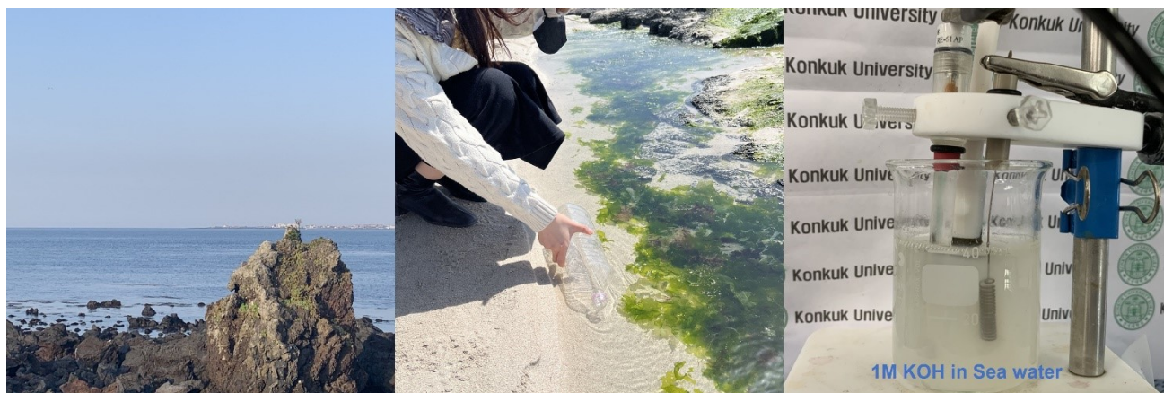
Figure S22. Photographs of natural seawater of Gimnyeong sea in Jeju island, Korea and 3 electrode cell for OER measurement in 1M KOH with sea water.
