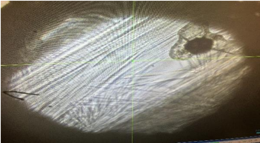
Figure S1.7: Image of TFE within the DAC after 2 nd pressure increase, the TFE crystal form changed to needles. Sample pressure found to be 0.71(5) GPa
