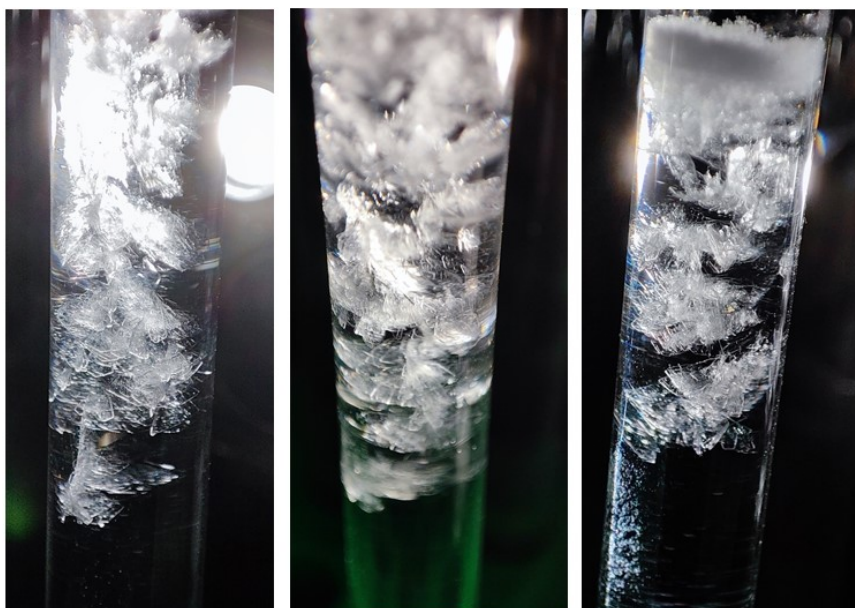
Fig. S7 Optical graphics of \text{Sn}(\text{SC}_n\text{H}_{2n+1})_4 single crystals grown by a layering diffusion method in \text{CHCl}_3/\text{EtOH} . From left to right are \text{Sn}(\text{SC}_{12}\text{H}_{25})_4 , \text{Sn}(\text{SC}_{14}\text{H}_{29})_4 and \text{Sn}(\text{SC}_{16}\text{H}_{33})_4 .
