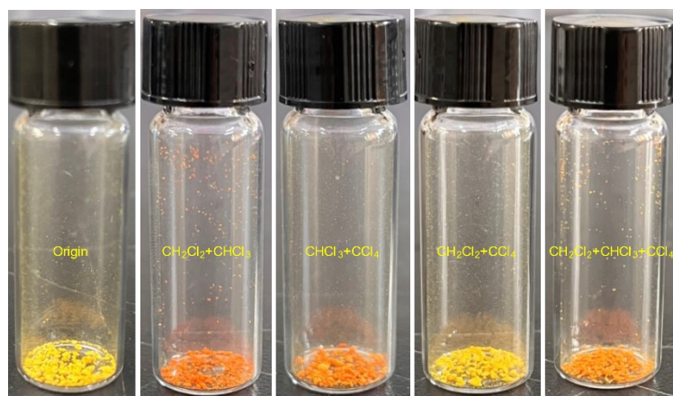
Figure S10. Photographs showing the color changes of crystalline DHTA-cage 1 upon exposure to equimolar mixtures of biphasic or tertiary solvent vapor.
