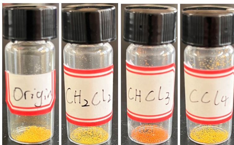
Figure S7. Photographs showing the color changes of crystalline DHTA-cage 1 upon exposure to halogenated methane (CH 2 Cl 2 , CHCl 3 and CCl 4 ) vapor.
