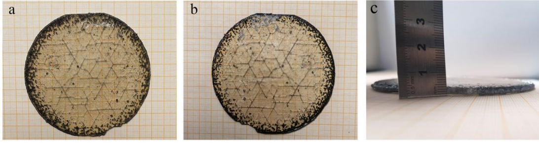
Fig. S4 (a) Ga surface grown on HMGA substrate to obtain GaN single crystals, (b) N surface grown on HMGA substrate to obtain GaN single crystals, (c) GaN single crystal thickness is 3 mm.
